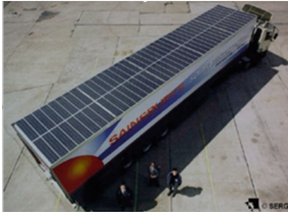
Fig. 4.3 Temperature-controlled vehicle with solar power (Reprinted by permission of http://prod.sandia.gov )
