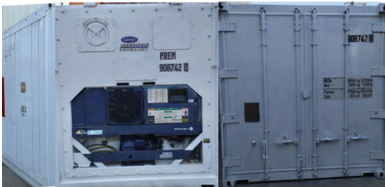
Fig. 4.8 Refrigerated container (integral)
