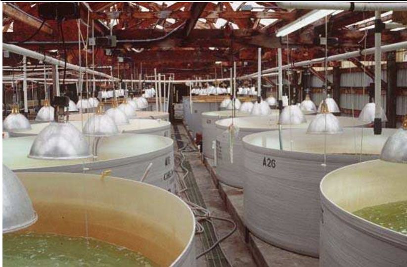
Figure 2.7.a. Batch culture systems for the mass production of micro-algae in 20,000 l tanks .
