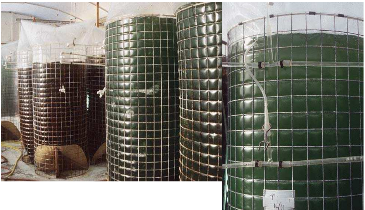
Figure 2.12. Continuous culture of micro-algae in plastic bags. Detail (right) shows inflow of pasteurized fertilized seawater and outflow of culture.
