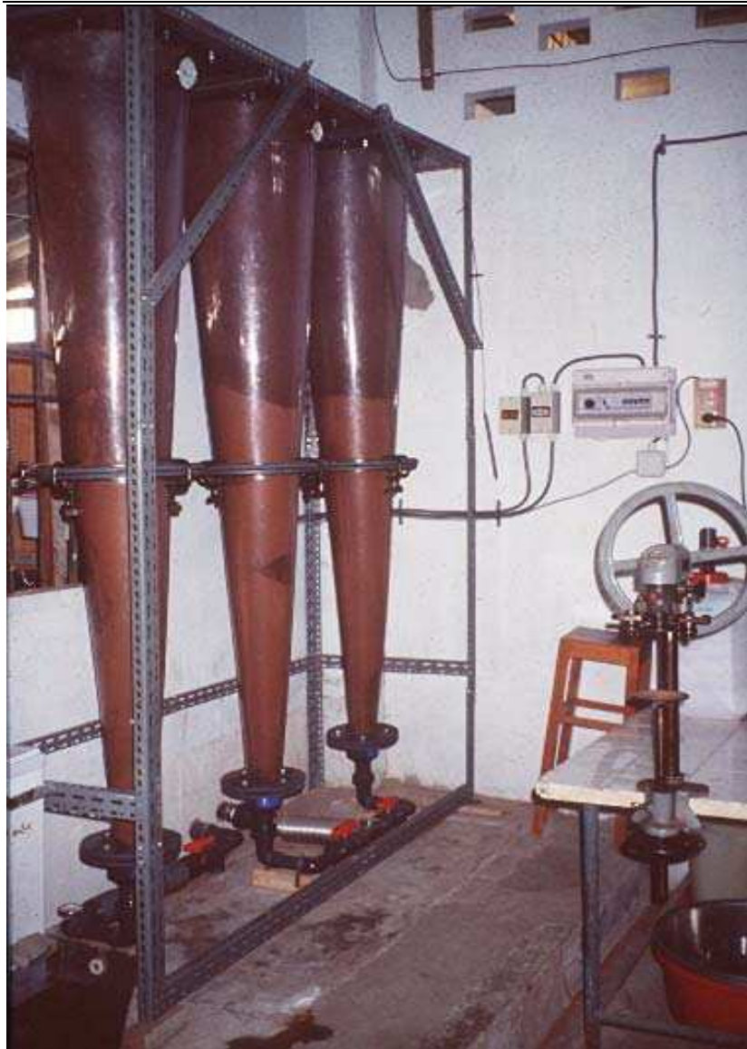
Figure 4.5.20. A fluidized bed dryer for Artemia cysts.
