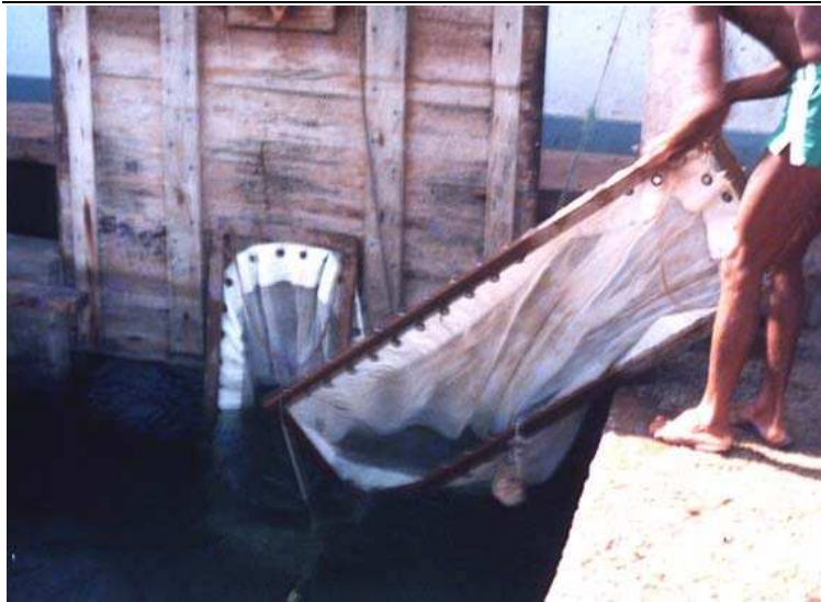
Figure 4.5.14. Installation of filter nets at the sluice gate for Artemia biomass harvesting in solar saltworks.
