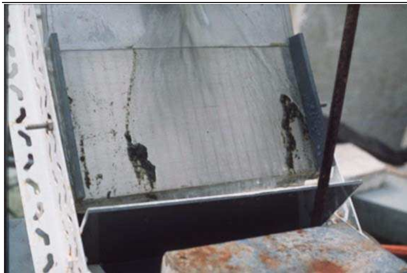
Figure 4.5.5. Close-up of welded-wedge filter screen and filtered zooplankton.
